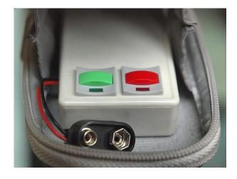
Inside the case there is a power connector, green power button combined with LED on/off indicator and red turbo mode button.
