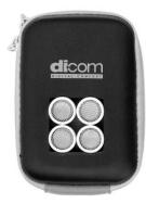
**SPYSONIC HANDHELD+** is a portable version of ultrasonic jammer of audio recorders with **ULTRANOISE** technology. The jammer is disguised as a camera case, dimensions (cm) 11x8x4. Number of ultrasonic transmitters: 4. Powered by Duracell - Duralock 9V that can last up to 5.5 hours in standard mode and up to 2 hours in turbomode.
